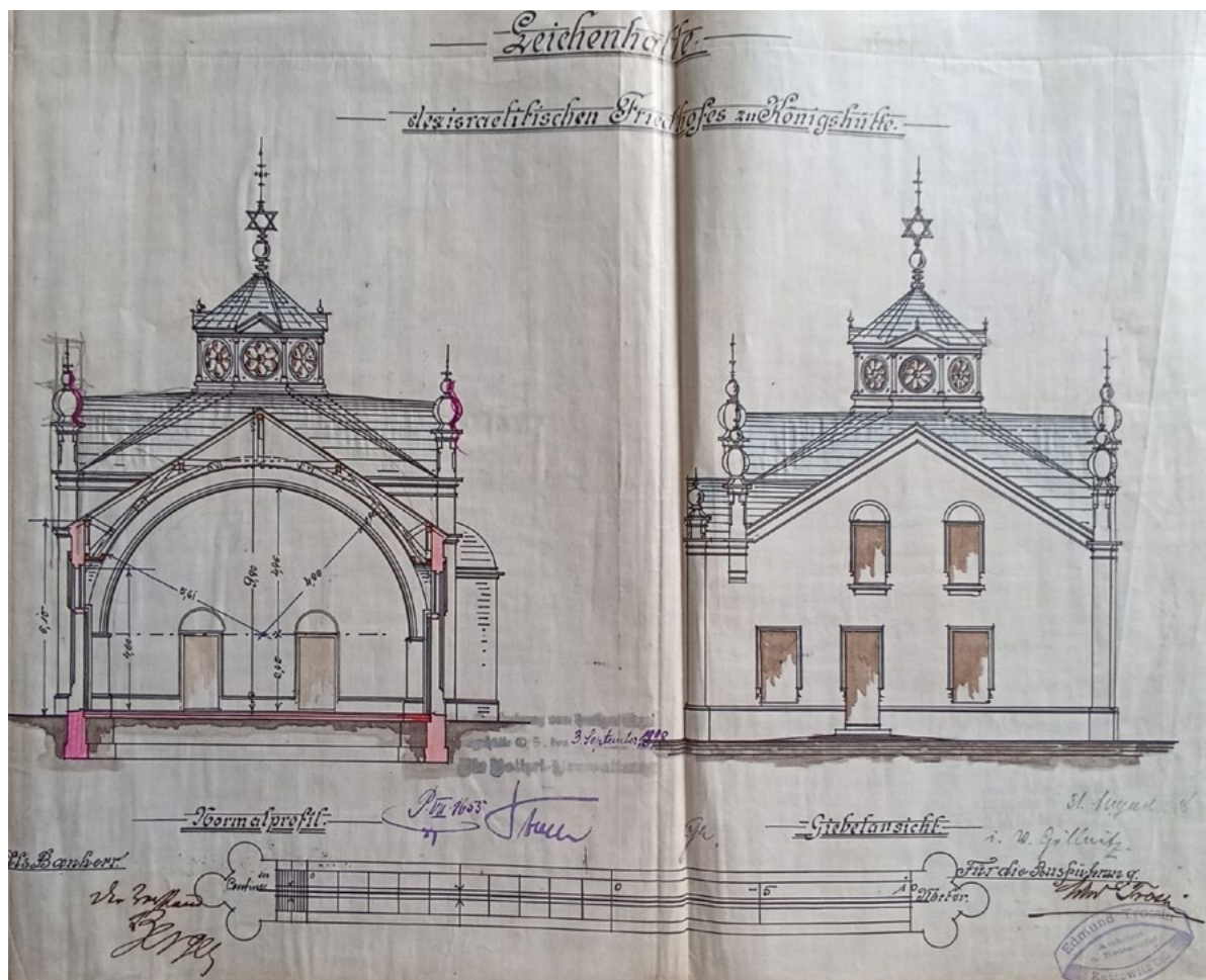
Fig. 3. Edmund Trossin, the design of the funeral home at the Jewish cemetery in Chorzów, 1898. The cross-section. The City Hall Archive in Chorzów.
