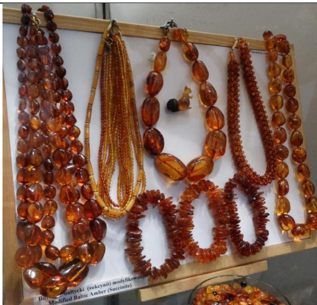
Fig. 20. Samples of the Baltic amber modified in an autoclave, which became transparent, darkened. Amber Laboratory by Gabriela Gierłowska, International Fair of Amber, Jewellery and Gemstones Amberif 2017. Photo: A. Peliński.
